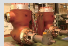
主蒸気弁 Main steam valve
