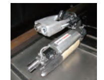
PCV ® 内部調査装置 02 Investigation device for pressure containment vessel
